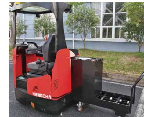
*Standard configuration: Battery side roll-out + trolley(optional)*
