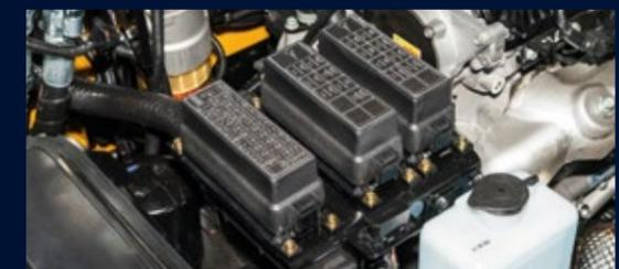
All fuses and relays are centralised in three boxes with **enhanced waterproof and dustproof protection IP65**. The boxes themselves are located under the engine hood for **quick access**.
