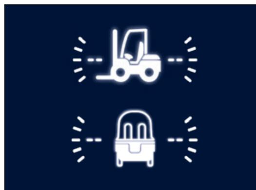
While driving the machine-control-unit (MCU) senses longitudinal and lateral movement and **alerts the driver if the preset stability values are exceeded.**
