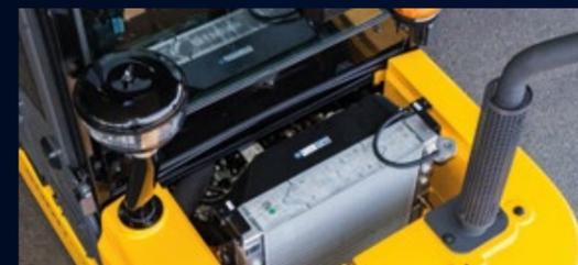
The radiator can be accessed by a removable top cover to **reduce the downtime when checking and refilling the coolant or cleaning the radiator**.
